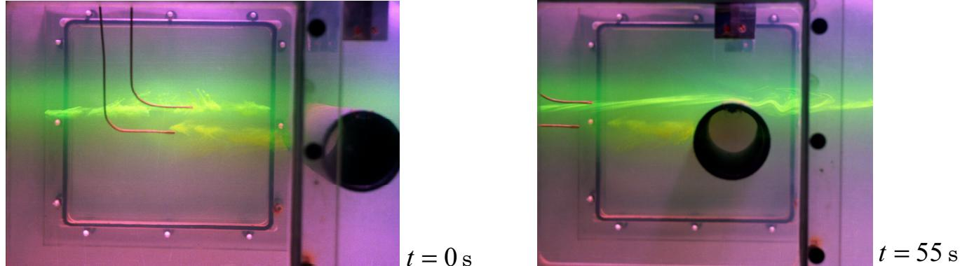
$D = 7.6 \text{ cm}$ ;  $T_b = 7.1 \text{ s}$ ; Dye and schlieren visualization  $D = 5.0 \text{ cm}$ ;  $T_b = 7.4 \text{ s}$ ;
